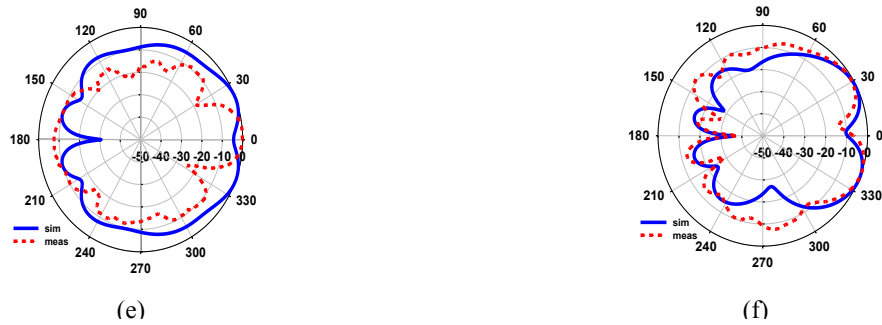
Figure 1: (a) Topology of the proposed antenna, (b) optimized diamond-shaped slotted AMC, (c) reflection phase of the optimized AMC unit cell, (d) reflection coefficient results, and radiation pattern in the yz-plane (e) at 2.45GHz, (f) at 5.8 GHz. The dimensions of the optimized antenna are L_a=90\text{mm} , W_a=90 , L_b=47 , W_b=62 , a=9 , b=34 , c=26 , d=4 , e=21 , f=2 , g=12 , h=2 . The dimensions of optimized AMC unit cell are L=30 , W=30 , L_1=27.85 , W_1=27.85 , \text{inner}=10.55 and \text{outer}=11.9 . All dimensions are in mm.
