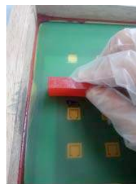
Figure 5: The squeegee rubber must be in the incline position, the angle of 45°.
