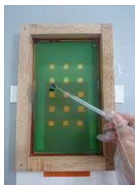
Figure 4: The graphene ink is ready to be printed on Kapton film.
