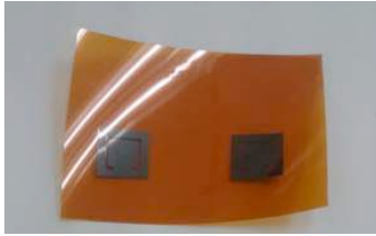
Figure 7: Grey colour appeared after the graphene ink antenna being cured.
