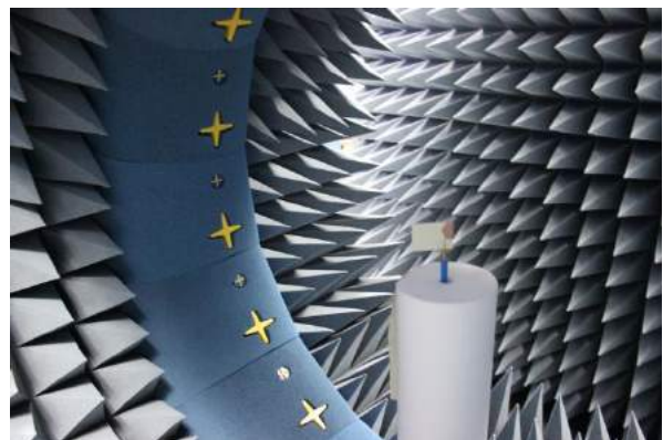
Figure 5: Antenna measurement in Satimo nearfield measurement system.
