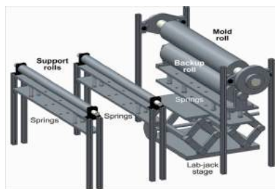
Figure 3 3D CAD drawing of an imprinting module; the mold roll and backup roll are responsible for pressurized imprinting, while the support rolls help secure uniform and continuous substrate feeding.
