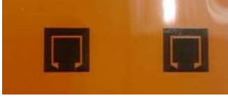
Figure 6: The antenna pattern made by graphene ink are printed on Kapton film substrate.
