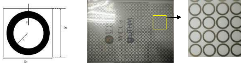
Fig 1. (a) Unit cell of the designed single ring loop FSS; D_x = D_y = 10.75 mm, R_1 = 4.2 mm; R_2 = 4.9 mm; (b) Fabricated FSS on PET substrate.
