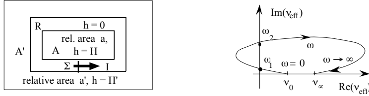
Fig. 4 Left: Horizontal cross section of C . The ring current I is H - H' (by Ampère), one has I = i\omega CV , where V is the voltage drop across the gap, and V relates to H by Faraday. Hence the formula for v_{\text{eff}}(\omega) given below. Right: Plot of v_{\text{eff}} in the complex plane, parameterized by the angular frequency, if Joule losses are accounted for.
